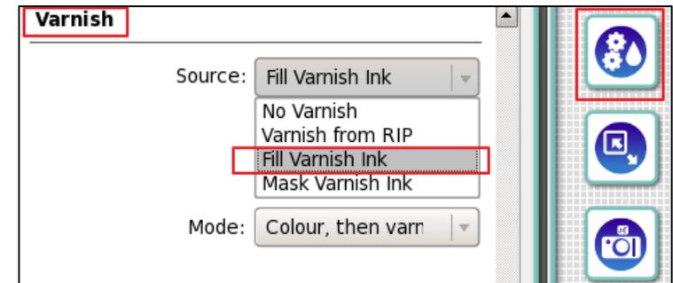
Alternatively Jeti engines are also capable of creating masked varnish layer, which will jet a varnish ink on top of every pixel that has a CMYK different from 0 0 0 0. On Asanti this option can be selected as “Mask Varnish (on Printer)”.
