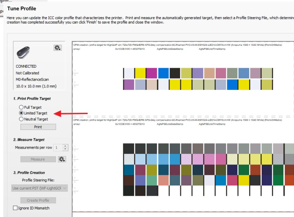
*There are 3 target options for profiling: “Full Target”, “Limited Target” and “Neutral Target”. The limited target will print a smaller strip. The measured results are combined with the original profile into a new tuned profile. A full target will print the same target as used for the original profile. The profile is then generated from scratch. Advantage: more exact profiles. Disadvantage: a lot more work to measure (especially with a handheld device). The “Neutral Target” is explained below.*
