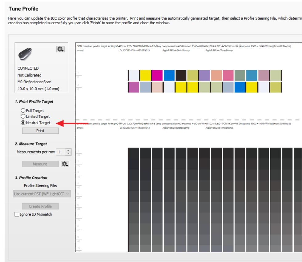
7. A successful measured row will receive a green check mark (minimal amount of measurements reached depending on value set in left pane). Notice the sound generated when a row is measured (different if successful or not). Useful when measuring strips printed on large substrates.
