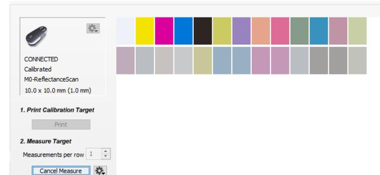
8. A successful measured row will receive a green check mark (minimal amount of measurements reached depending on value set in left pane). Notice the sound generated when a row is measured (different if successful or not). Useful when measuring strips printed on large substrates. It's advised to measure each wedge 2 times. Measurements can be deleted or exported by context clicking at the target.
