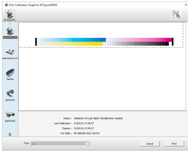
A QMS calibration job (order number: QMS – job name: [Ink Table] Calibration (QMS ID) will automatically be generated (this job will be deleted automatically after printing). The Calibration strip will be printed, dried and automatically measured by the online SpectroProofer. Even the ink table will be updated without any manual action required.
